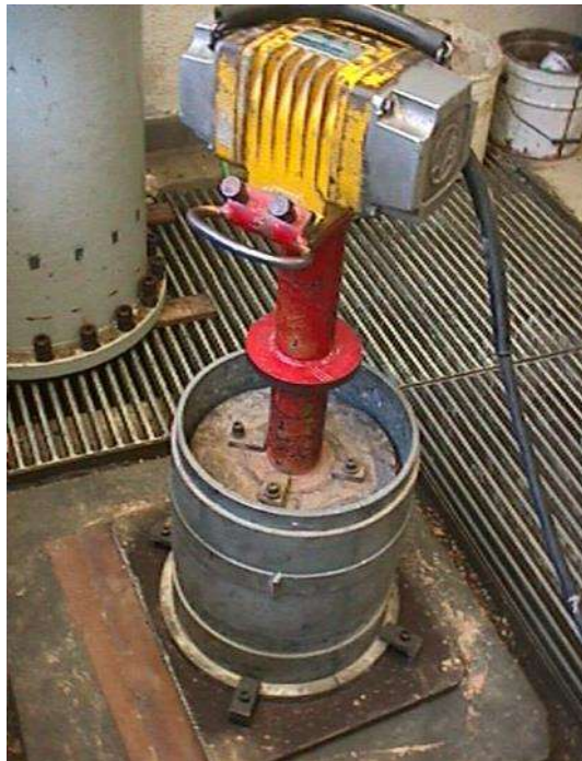
Figure 3.2 – Vibratory hammer in use during specimen compaction
