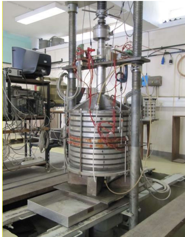
Figure 3.1 – DU50 cell assembled and in testing position at the loading frame
