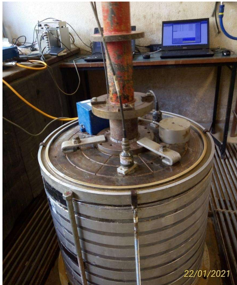
Figure 3.3 – View of the cell with the rigid plate and vibratory hammer at the top, and measuring devices
