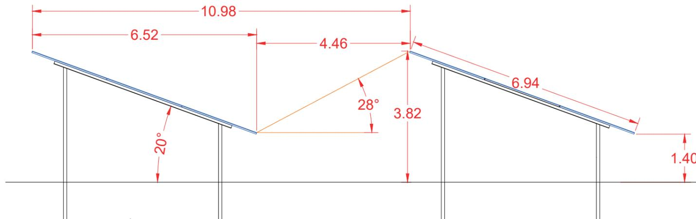
SCHÉMA D'IMPLANTATION DES STRUCTURES PHOTOVOLTAÏQUES
